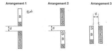
In Arrangement 1, Magnet B experiences a repulsive force of 5 N upwards.
