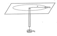
An experiment is performed using the apparatus above. A small disk of mass  $m_1$  on a frictionless table is attached to one end of a string. The string passes through a hole in the table and an attached narrow, vertical plastic tube. An object of mass  $m_2$  is hung at the other end of the string.
